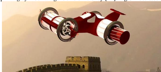
FIGURE 6 iCar Magnus-effect-based car-plane [14]
