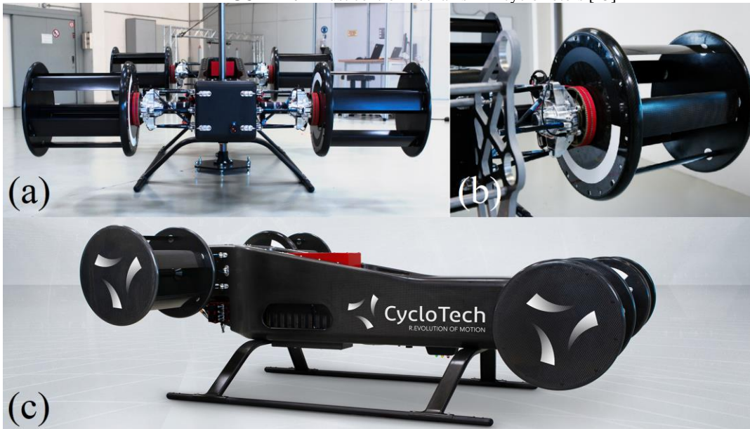
FIGURE 11 Thrust control mechanism in cyclo-rotors [25]
