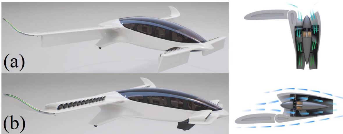
FIGURE 15 Tilting mechanism of Lilium (a)vertical take-off and landing (b)cruise mode [33]
