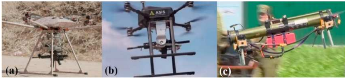
Fig. 115. Views of armed military quadrotors, (a) Duke Robotics military quadrotor [342], (b) Turkey's armed quadrotor [343], and (c) RPG-combined quadrotor [344].
