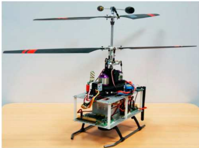
Fig. 105. The mono-rotor developed by Wang et al. for SAR missions [310].
