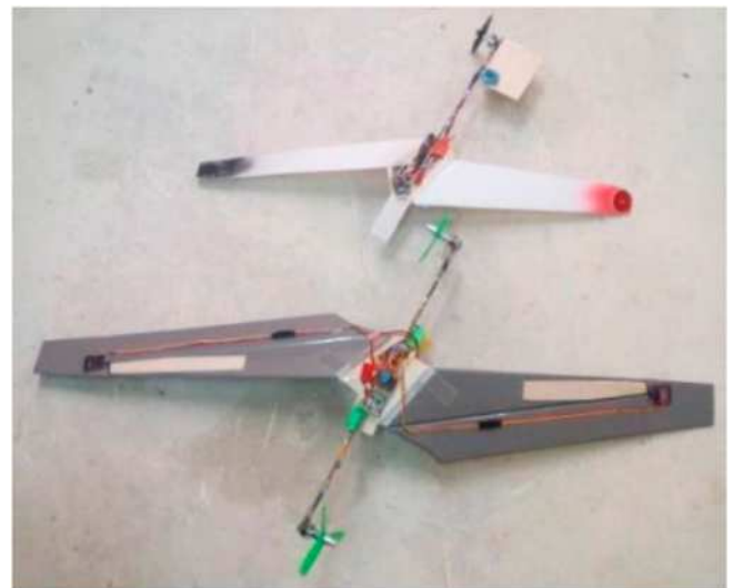
Fig. 44. An example of a two-wing rotor UAS [158].
