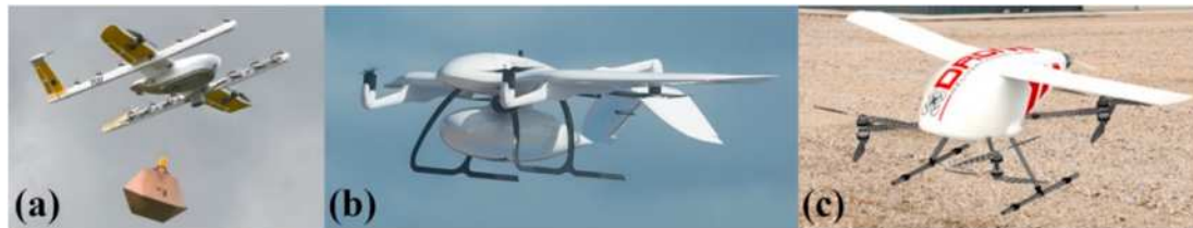
Fig. 113. Views of hybrid delivery drones; (a) Google X's dual system drone [333], (b)Wingcopter's tilt-rotor drone [334], and (c) DDC's dual system drone [336].
