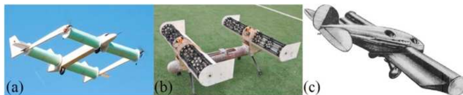
Fig. 15. Examples of Magnus-effect UASs (a) four Magnus wing with the rough surface [56], (b) four Magnus wing with blades [57], and (c) Gligorin's concept of combined fixed-wing and Magnus rotor [52].
