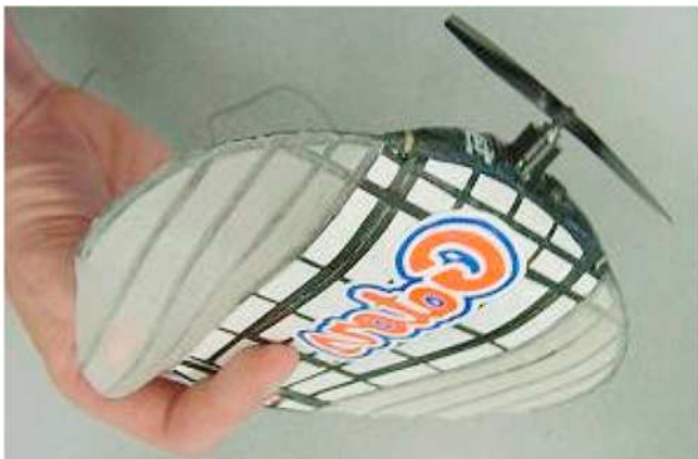
Fig. 10. The morphing wing MAV developed by Ifju et al. [50].
