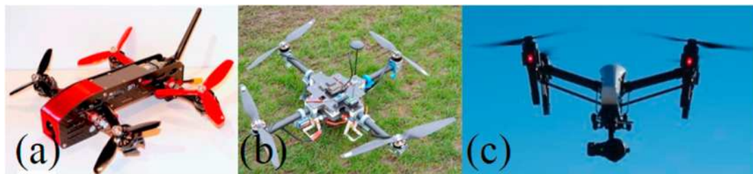
Fig. 31. Views of (a) XRay tilt-rotor quad DIY ARF FPV [116], (b) Tilt-rotor quadrotor designed by Ben Junaaid et al. [115], and (c) Inspire 1 Pro tilt-rotor quadrotor developed by DJI [117].
