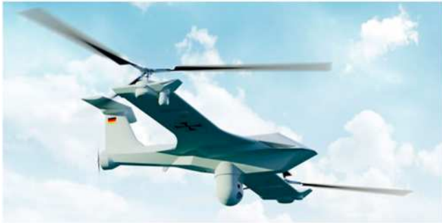
Fig. 76. The dual system UAS combines the capabilities of an aircraft and helicopter to provide a wide range of missions, developed by Airborne [214].
