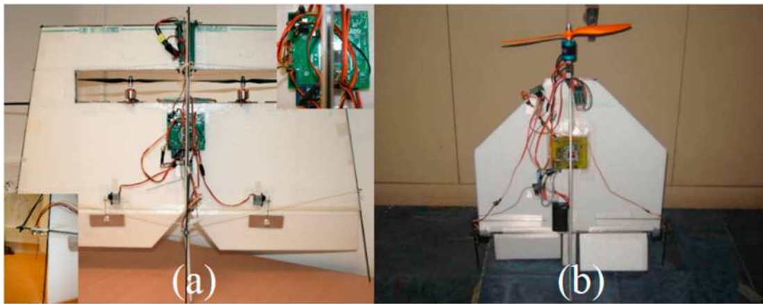
Fig. 60. Views of semi-tail-sitter designed by (a) Ta et al. [189], and (b) Garcia et al. [188].
