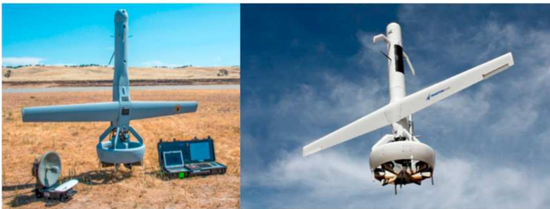
Fig. 54. Ducted-fan tail-sitter, developed by MartinUAV company [178].
