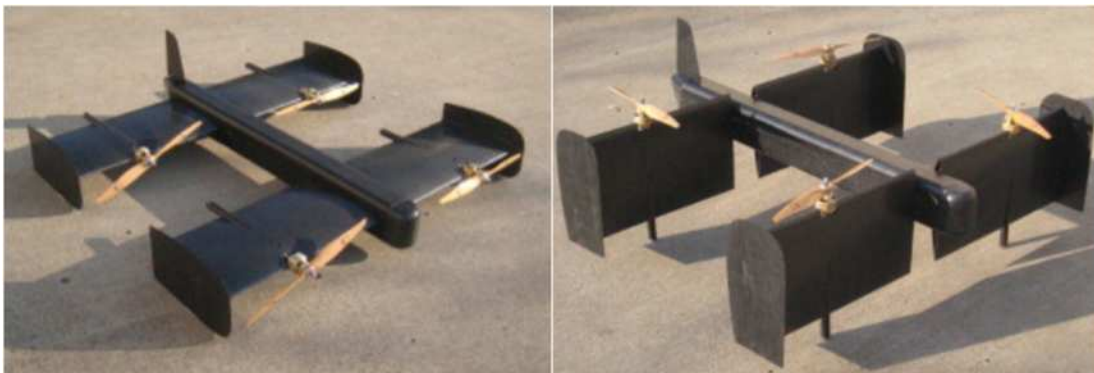
Fig. 68. Tilt-wing drone developed by Cetinsoy et al. [204].
