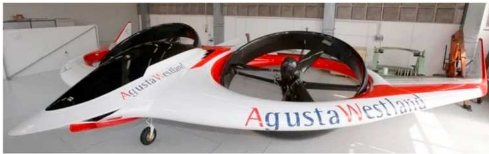
Fig. 63. Tilt-rotor drone developed by AgustaWestland [194].
