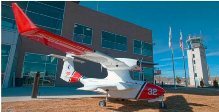
Fig. 108. DroneAmerica's fixed-wing firefighting UAS [317].
