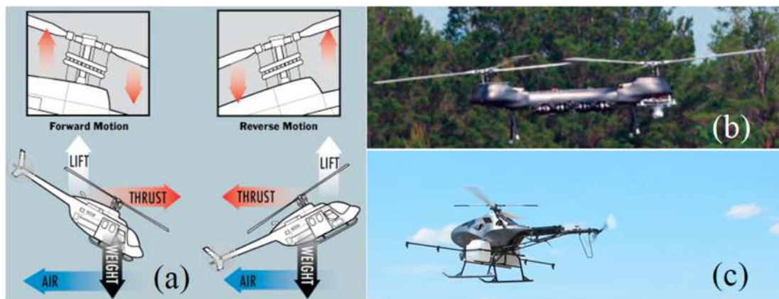
Fig. 41. View of (a) swash-plate function [149], (b) unmanned tandem-rotor helicopter developed by DPI UAV Systems [85], and (c) SY260H coaxial unmanned helicopter [150].
