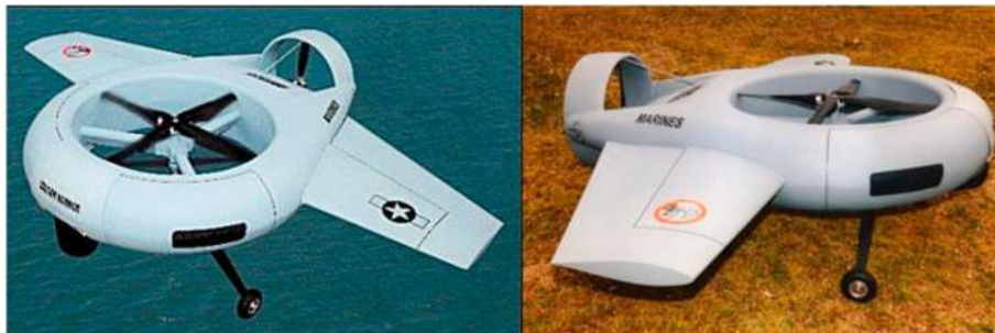
Fig. 73. Hybrid drone with dual systems developed by Sikorsky [84,210].
