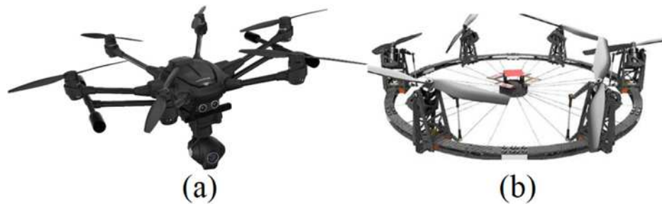
Fig. 35. Views of (a) Typhoon H hexarotor developed by Yuneec [125], and (b) a tilted-rotor hexarotor developed by Ryll et al. [126].
