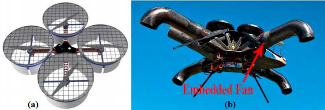
Fig. 29. Views of (a) Ducted-fan quadrotor developed by Rones [106], and (b) ducted quadrotor drone with embedded fans developed by Rivellini [107].
