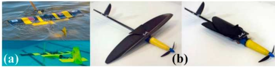
Fig. 121. Views of underwater HTOL drones; (a) fixed-wing underwater drone developed Weisler et al. [360] and (b) morphing wing underwater drone developed by Siddall et al. [361].
