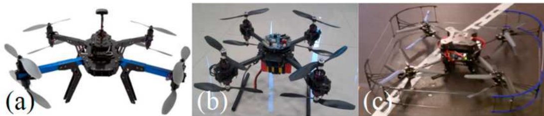
Fig. 30. Views of coaxial quadrotors developed by (a) Tashreef et al. [110], (b) Haddadi and Zarafshan [109], and (c) Saied et al. [111].
