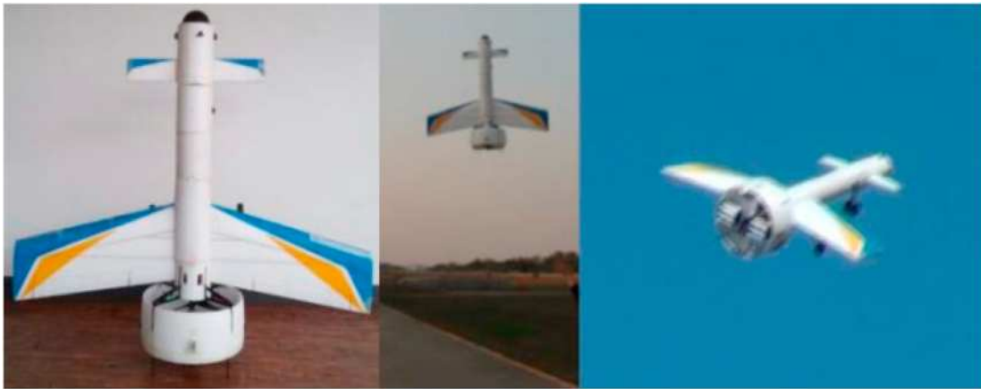
Fig. 53. Ducted-fan tail-sitter, developed by Jung et al. [177].
