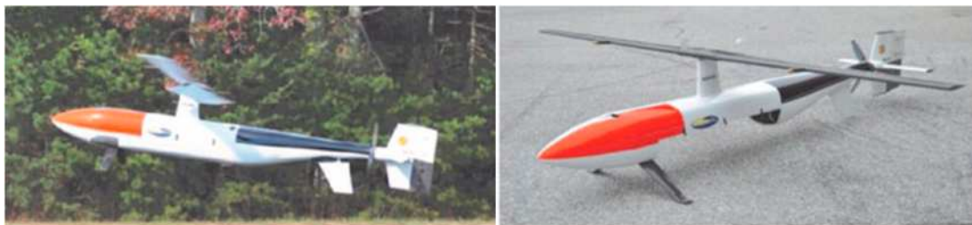
Fig. 77. Views of NLR The stop-rotor rotary-wing drone [215].
