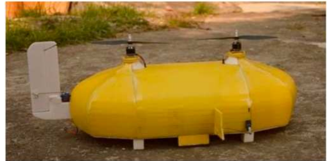
Fig. 37. Views of Coanda-effect UAS developed by Haque et al. [132].
