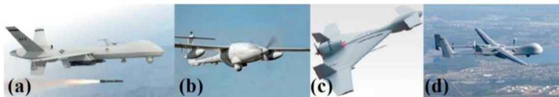
Fig. 114. Views of different fixed-wing military UASs, (a) V-tail [338], (b) T-tail [339], (c) delta wing [340], and (d) twin tail boom [341].
