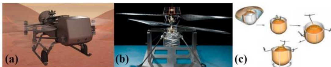
Fig. 127. Views of multirotors drones for space missions; (a) NASA's Dragonfly for Titan exploration [372], (b) NASA's coaxial mono-rotor drone for Mars explorations [373], and (c) tri-rotor drone designed by Young et al. [384].
