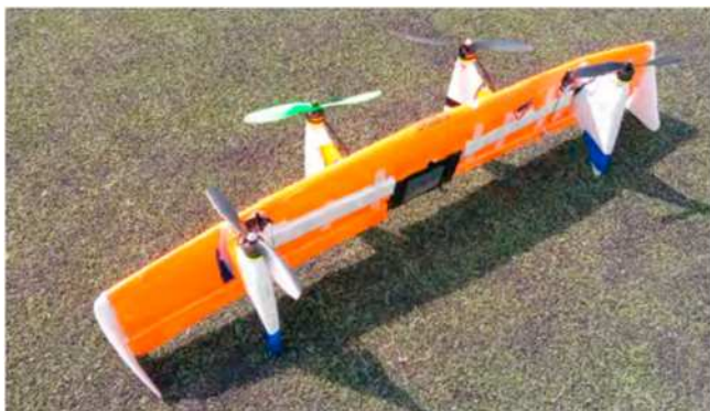
Fig. 59. Semi-tail-sitter, developed by Reyes [187].
