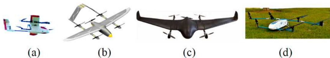
Fig. 98. Dual system hybrid UASs for mapping and inspection missions; (a) V-TOL Aerospace Goshawk Hybrid [275], (b) South Skycruiser MF2500 [276], (c) DeltaQuad Pro [277], and (d) HAMR's unconventional dual system hybrid UAV [278].
