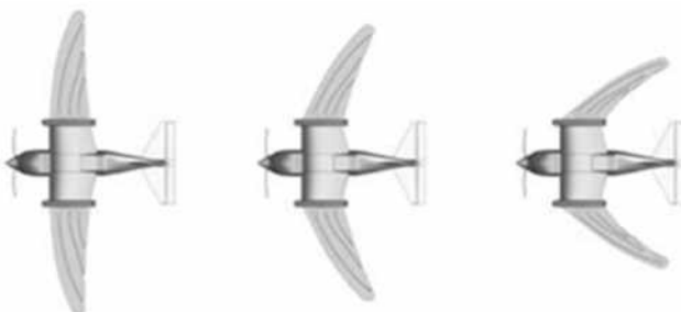
Fig. 8. Fixed-wing with a variable-sweep angle [48].
