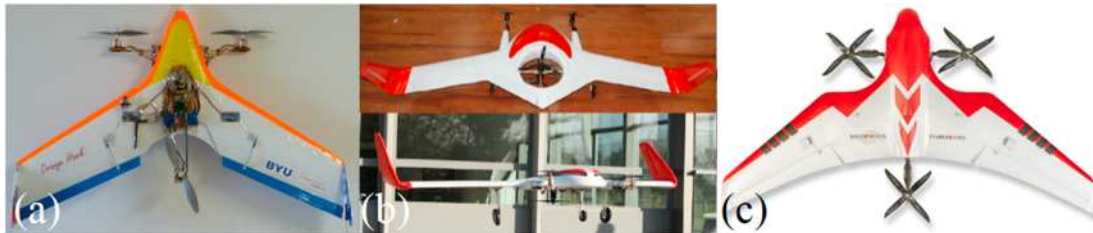
Fig. 64. Views of tilt-rotor drones designed by (a) Carlson [195], (b) Aktas et al. [196], and (c) BirdsEyeView Co [197].
