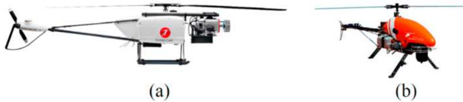
Fig. 96. Unmanned helicopters developed for mapping and inspection missions; (a) Flying-Cam SARAH [267] and (b) SNIPER UAV Helicopter [268].
