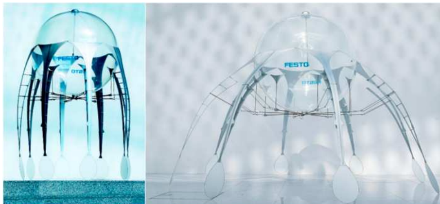
Fig. 86. Views of Jellyfish-inspired UAS developed by Festo [234].
